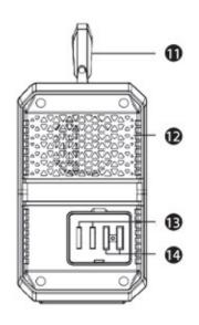
1. AC output port×2 6. AC indicator light 11. Easy-carry handle 2. DC power button 7. AC power switch 12. Cool fan 3. Power indicator light×4 8. DC power indicator 13. Spare fuse tube×2 4. DC 15V input port 9. DC 12V output port×2 14. Fuse tube×2 5. USB indicator light 10. USB output port×4
