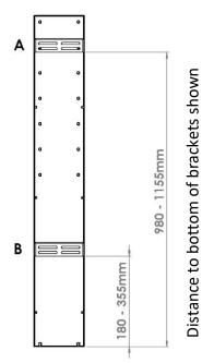
Position the column over the brackets, ensure the base of the column is resting on the ground. Then secure the column in place using the M8 bolts provided. Check that the column is vertical using a spirit level and make any necessary adjustments.
