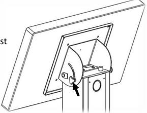
2. Whilst holding the screen in one hand pull out the plunger pin with the other hand and move the screen into the desired position, when in position release the plunger pin and allow it to snap into place.
