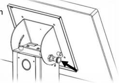
3. With the plunger in position the thumb wheel should now be tightened to prevent accidental movement of the tilt mechanism.
