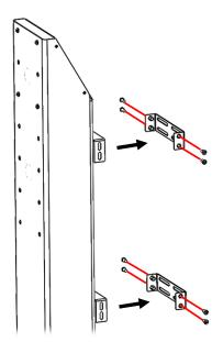
5. Remove the grommets from the front of the column. Then secure the mount in place using four M8\*20mm bolts, the mount can be bolted in 5 different positions and offers 400mm of height adjustment in 100mm increments.
