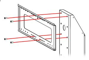
6. Fix the brackets to the back of the screen using fixings of an appropriate size and length for your screen. Ensure the brackets are as central as possible.
