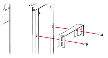
3. Using the technical drawing mount the wall mounts to the wall in the positions shown. Be sure to take into account the added height of the adjustable feet.
