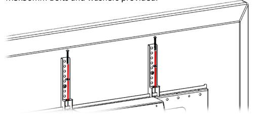
9. Unscrew the four M4 bolts and remove the rear cover. Pass power cables for the screen through the grommet on the front of the column and plug into the 4 way power strip. Once cabling is complete bolt the cover back in place.
