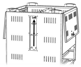
11. Pass the cables through the grommets in the central tray, make sure there is enough slack to reach your device. It is recommended to drop the shortest cables through the nearest grommet where possible.
