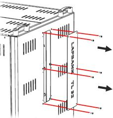
Unlock and open the laptop compartment doors. Remove the eight M5 bolts indicated then lift off the cover.
