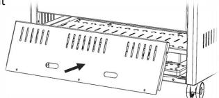
**B.** Secure the hatch using the three M5 fixings removed in step 1.
