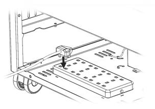
the sockets, if possible unplug the mains lead from the transformer.
