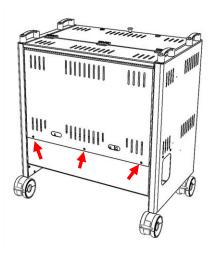
2. Open the hatch around 45 degrees and unhook the hatch from the trolley.
