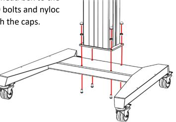
3. Secure the mount to the headbox using four M8 bolts.
