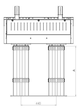
2. With the four brackets fixed to the wall move the heavy duty lift up to the brackets and check the alignment of the brackets with the columns. If the columns align with the brackets use the U-Shaped straps to secure the lift to the wall as shown in the diagram. Each strap should be secured with four M8 bolts.
