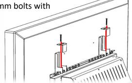
4. To access the integrated 4-way power strip in the headbox, unscrew the three fixings indicated and lift off the vanity cover.
