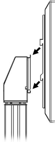
6. Secure the screen in place by fixing through the brackets into the mount plate, use the M5x50mm Bolts and washers provided.
