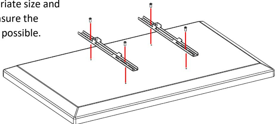
5. Hook the screen onto the mount rail.
