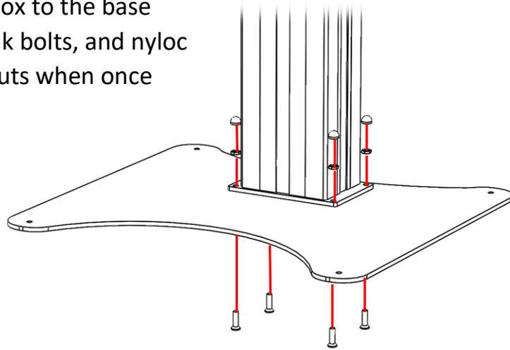
2. Secure the mount to the headbox using four M8 bolts.
