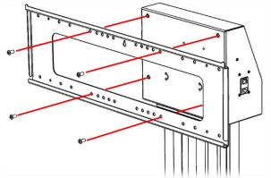
3. If required the base can be bolted to the floor for extra stability.
