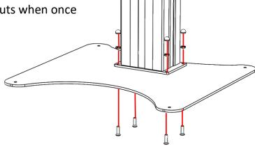
2. Secure the mount to the headbox using four M8 bolts.
