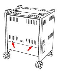
2. Open the hatch around 45 degrees and unhook the hatch from the trolley.
