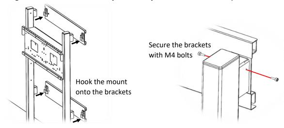
11. Attach the hangers to the back of the screen.
