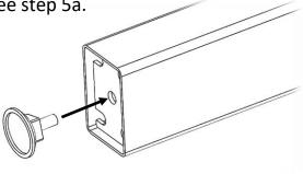
5a. Secure the extensions in place using a M10 bolt, then thread in the adjustable foot and push the cover into place.
