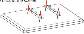
12. Hook the screen onto the mount rail.
