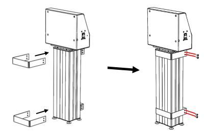
7. Fix the mount plate to the headbox using four M8 bolts.
