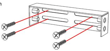
6. Move the column up against the two brackets on the wall, then slide the U-shaped part of bracket around the column and secure in place using four M8 bolts for each bracket.
