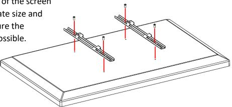
9. Hook the screen onto the mount rail.
