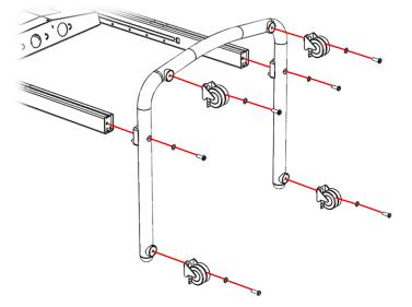
8. Use four M6 bolts to bolt the mount plate to the trolley.
