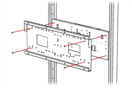
9. Attach the hangers to the back of the screen, make sure the hangers are as central as possible.
