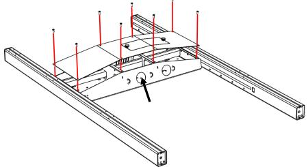
6. Attach the handle using the bolts you put aside in step 3 and the bolts already fitted in column. Use the top set of holes. Add the 16 caps into the holes indicated
