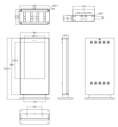
Note: The Ø30 holes are for access, we recommend using M10 anchor bolts that will fit into the Ø16 holes.
